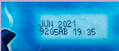
FIG 3. Typical low-resolution coding and marking print.
