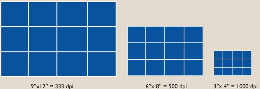
FIG 21: The same 12-megapixel (4000x3000px) image placed on the page at three different sizes.
