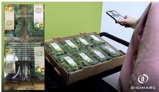
FIG 2. Traceability can be enabled using unique, serialized identities on product packaging and labels
