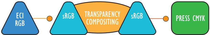
FIG 24: Color transformations with transparency requires significantly more processing.
