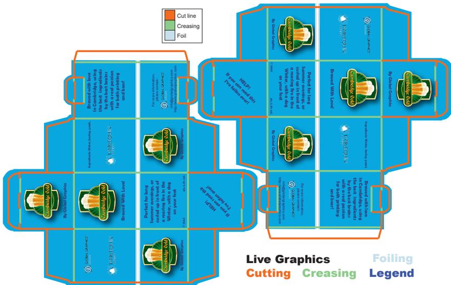
FIG 38: Common technical marks for a premium folding carton.
