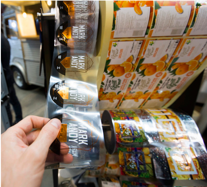
Fully variable printing: The Digital Series HD can print thousands of labels per minute, and each label can be different and at variable places on the web.
